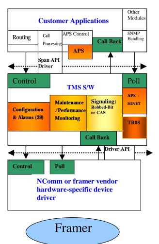
Functionally, drivers do not process data or make high-level decisions (That's where TMS adds tremendous value). Drivers are framer (hardware) specific. The NComm drivers provide the same API for all vendor framer devices within a technology (T1, etc.). These drivers accommodate device differences and nuances. By the time you get to the top of the driver, all framers are the same to applications above it. Thus, code written to the NComm Driver API will talk to any framer device.
