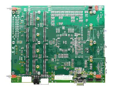
NComm's Manchester card allows NComm's Telecom Interface Modules (TIM) to be used under the Windows Operating system. TIMs provide the hardware interface to T1, E1, T3, E3, SONET/SDH, ISDN and timing networks. Using the Microsoft Windows Operating system and the Manchester card Microsoft Windows based system can be debugged and tested before system hardware is designed and available.
